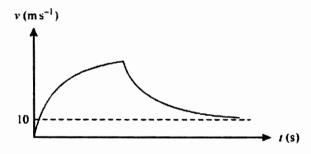
The diagram shows a (t, v) graph for the parachutist's motion, as modelled using the above differential equation.
