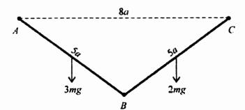
Two uniform beams AB and BC, each of length 5a, have masses 3m and 2m respectively. The beams are freely jointed to fixed points at A and C, and to each other at B. The points A and C are on the same horizontal level at a distance 8a apart, and the beams are in equilibrium with B vertically below the midpoint of AC, as shown in the diagram.
