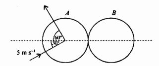
Two uniform smooth spheres A and B, of equal radius, are free to move on a smooth horizontal table. The mass of B is twice the mass of A. Initially B is at rest and A is moving with speed  $5 \,\mathrm{m \, s^{-1}}$ . The spheres collide, and immediately before impact the direction of motion of A makes an angle of  $30^{\circ}$  with the line of centres. After the collision A moves at right angles to its original direction (see diagram). Show that
